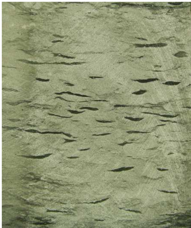
Figure 5.14 High-density of Nereites missouriensis in offshore-transition deposits illustrating an example of non-constrained textural heterogeneities. Presence of this ichnofabric promotes gas and light oil transmissivity in low permeability reservoirs in many fields in North America. Upper Devonian–Lower Mississippian, Bakken Formation, Saskatchewan, Canada. Core width is 9.5 cm. See Angulo and Buatois (2009).
